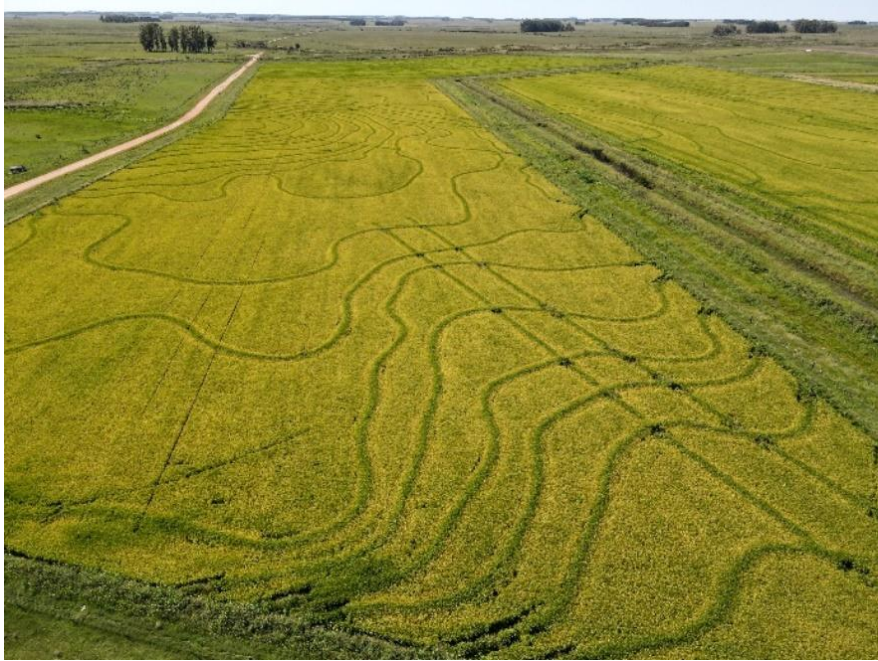
Figure 7: Photograph of a closely-spaced levee leveling system traditionally used for rice production on lowland soils in Uruguay and Southern Brazil.
