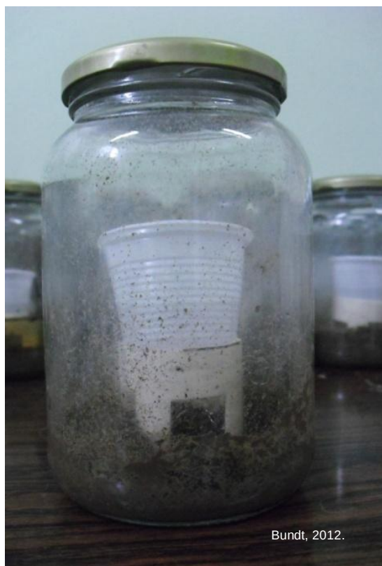
Figure 14. Chamber of C-CO 2 capture, used in the experiment of imidazolinone degradation in response to application history.
