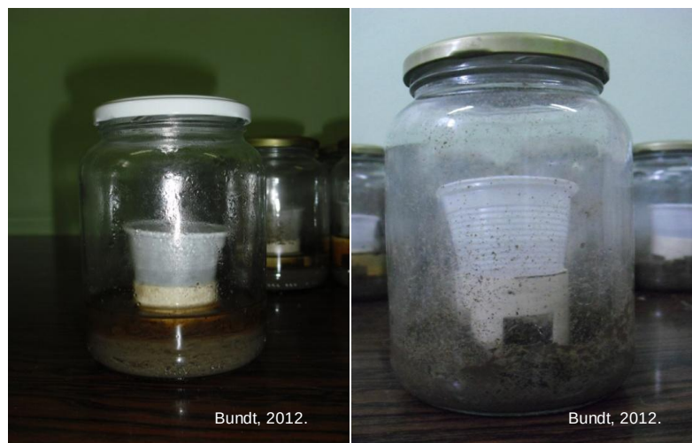
Figure 12: Chambers of C-CO 2 capture, used in the experiment of effect of temperature and soil moisture on degradation of imidazolinone herbicides.
