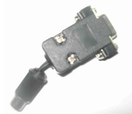
Figura 24: Interface serial 1-Wire
