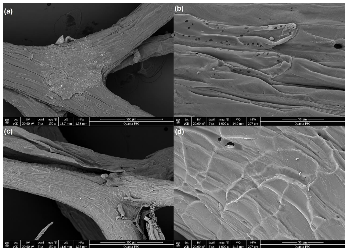
Figure 3-1.2: Images obtained by SEM images (at different magnifications) for (a,b) LF and (c,d) LF-g-PEI.
