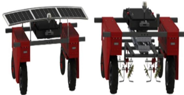
Figura 27 – The Digital Farmhand. Plataforma com painel solar.
