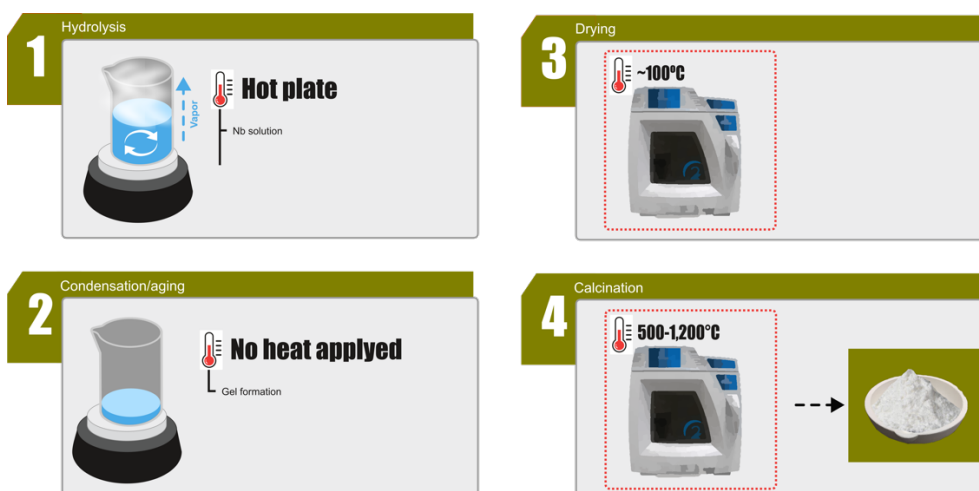
Fig. 5: Production of \text{Nb}_2\text{O}_5 using the sol-gel method.
