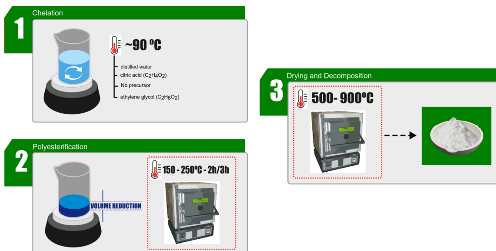
Fig 6: Generic graphical methodology of the Pechini method.
