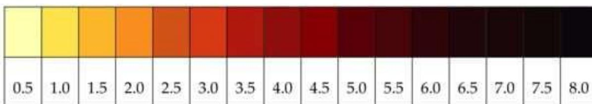
Figura 7- Escala de cor conforme a norma ASTM D1500.
