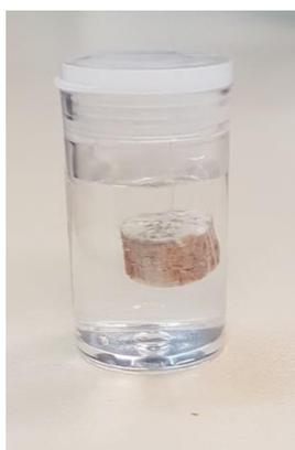
Figura 9 – Amostra imergida no SBF.
